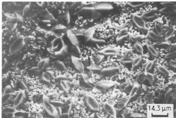
Figure 3 Surface microstructure after 150h cyclic exposure at 871 °C.
