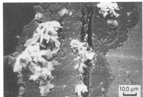
Figure 9 The microstructure after 16 h cyclic exposure at 1093 °C: the melt within the scale absorbed water from humid air to recrystallize. The crystal morphology is subject to change with time.
